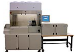
An on-site system screens letters and packages for the biological threat of anthrax. The technology is polymerase chain reaction, which detects the presence of anthrax spores and provides results by analyzing the DNA of an organism. Photo courtesy of Smiths Detection
